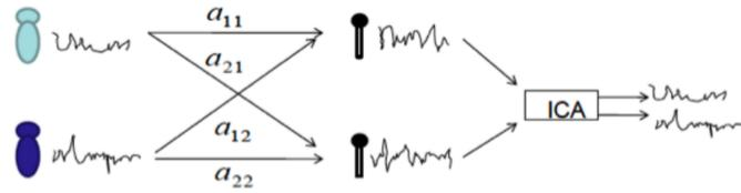
**Independent component analysis (ICA)** is a signal processing method for separating a multivariate signal into additive subcomponents with the assumption that the subcomponents are non-Gaussian and are statistically independent.
